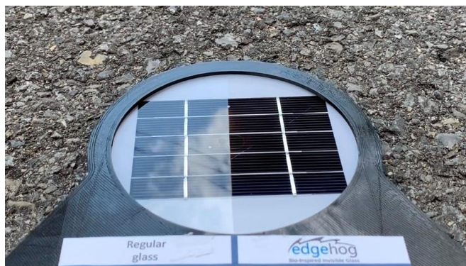
Figure 2 (right picture) – Here, the same glass substrate shown in Figure 1 is mounted on a solar cell. The left half, conventional glass, shows the reflection of the sky (wasted energy). The right half appears black appearance because all light is transmitted into the solar module and converted into electricity.
